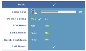
**LAMP HOUR**—Displays the operating hours since the last lamp timer reset.
